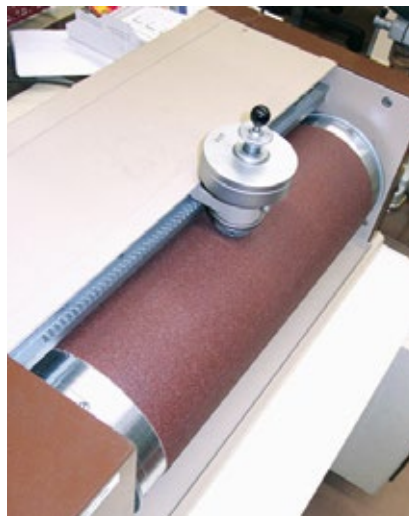
Test against abrasive paper.
