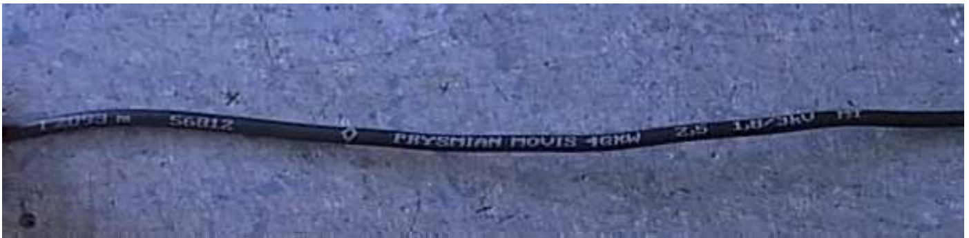
CABLE MARKING : 1 METER MARKING 56812 PRYSMIAN MOVIS 4GKW 2,5 1,8/3KV MT
