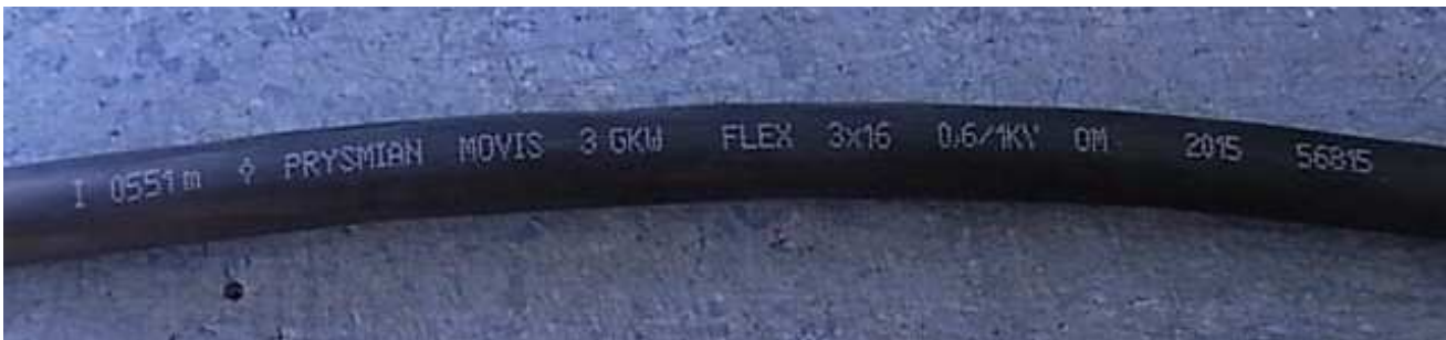
CABLE MARKING : PRYSMIAN MOVIS 3 GKW FLEX 3X16 0,6/1 KV OM 2015 I METER MARKING
