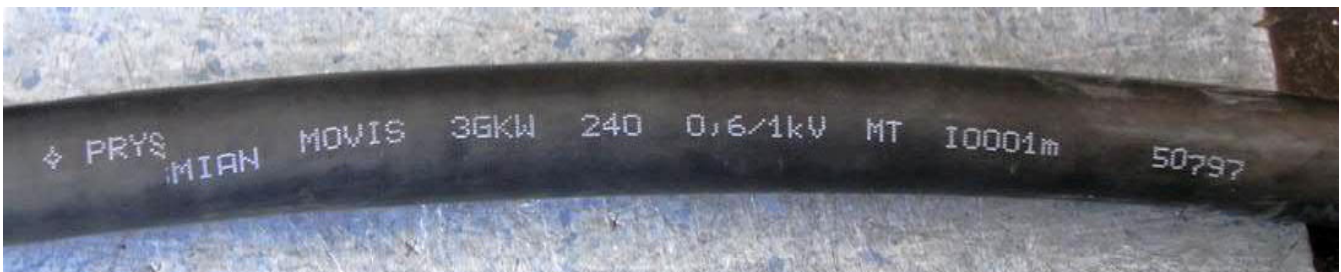
CABLE MARKING : PRYSMIAN MOVIS 3 GKW 240 0,6/1KV MT I meter marking 50797
