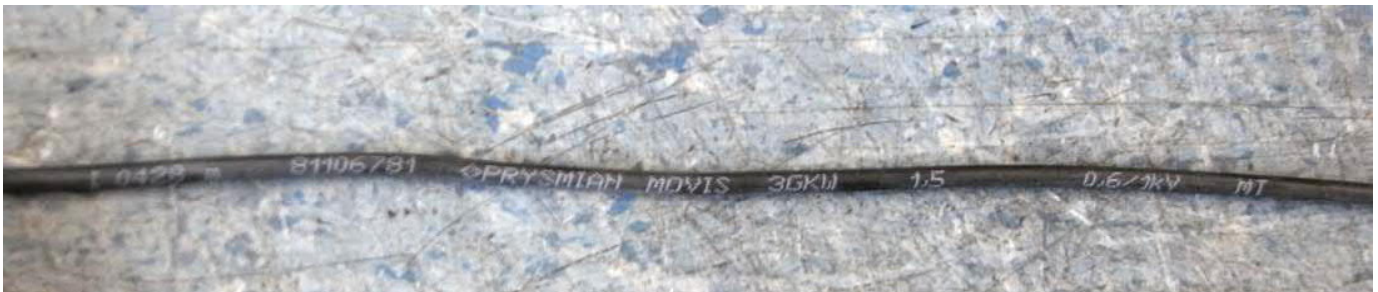
CABLE MARKING : I METER MARKING 81106781 PRYSMIAN MOVIS 3GKW 1,5 0.6/1KV MT
